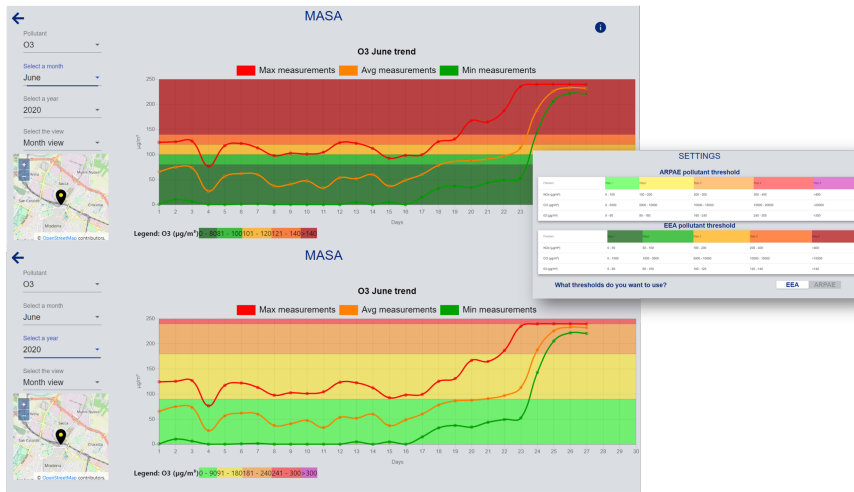
Fig. 9 Two month views for O_3 in June 2020 in the city of Modena: the top view uses ARPAAE scale and the lower EEA scale. The figure shows also the settings page where scales can be modified.
