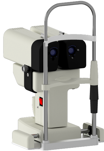
Figure 1. retinaWISE, a binocular silenced pupillometer equipped with three cameras allowing for simultaneous and bilateral pupil monitoring and two controlled light engines to generate silent substitution stimulation of the patient's eye fundus. An ophthalmic joystick and a chin rest are included to align the device with the patient's eyes.
