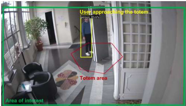
FIGURE 9. Snapshot of the prototype installed at Aitek facilities. The view is captured from the roof node camera. The green rectangle outlines the total area of interest, the red polygon defines the totem node area, and the yellow box marks the detected visitor.
