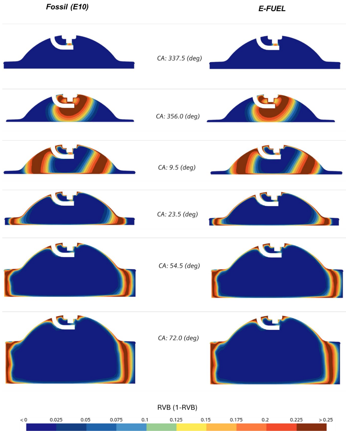
Figure 83 Comparison of flame development from a 3D-CFD perspective between fossil fuels and e-fuels.
