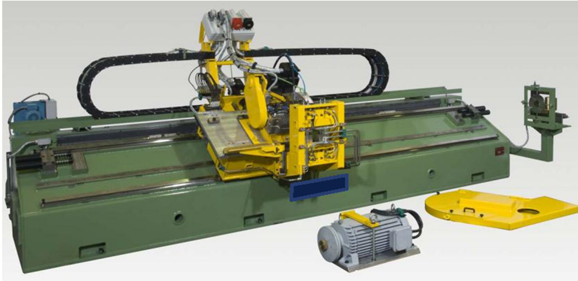
Figure 3.1: the Cut-off unit. The yellow part is the carriage which hosts the blade under study.
