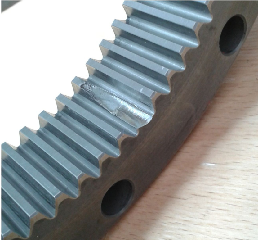
Figure 4.2: the damaged ring gear of the E50 stage.
