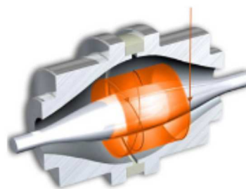
Fig.1.12 The operation of an Orbitrap mass analyser ( Http://www.thermoscientific.com , n.d.)
