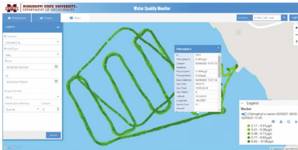
Figure 2.15: Map of the path followed by a floating drone during a monitoring mission (Source [7]).
