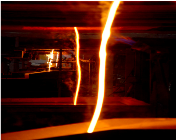
Figure 16. Quenching process to obtain the frit
