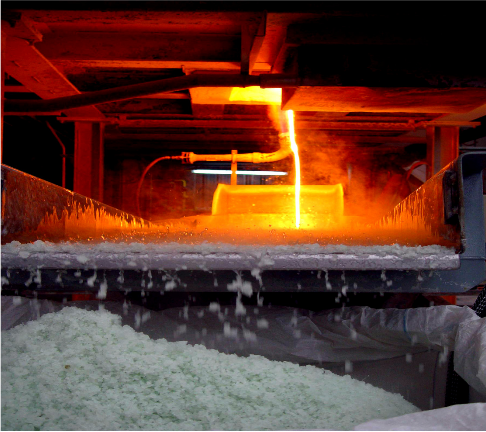
Figure 9. Frit glass during the cooling
