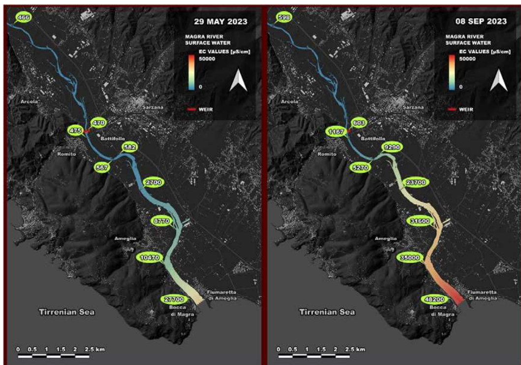
Figure 5 – At left: EC pattern representing the minimum SI observed along the R. Magra estuary. At right: EC pattern representing the maximum SI observed along the R. Magra estuary.
