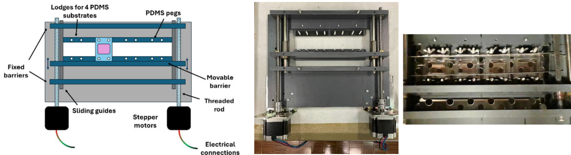
Fig. 47 Schematic representation and pictures of the multi-substrate uniaxial stretcher.
