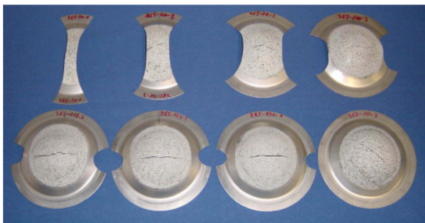
Fig. 5-3 – Example of fractured Nakajima formability test specimens
