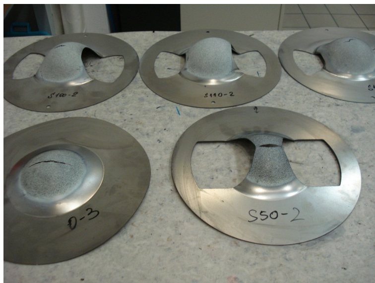
Fig. 5-9 – Nakazima specimens after testing
