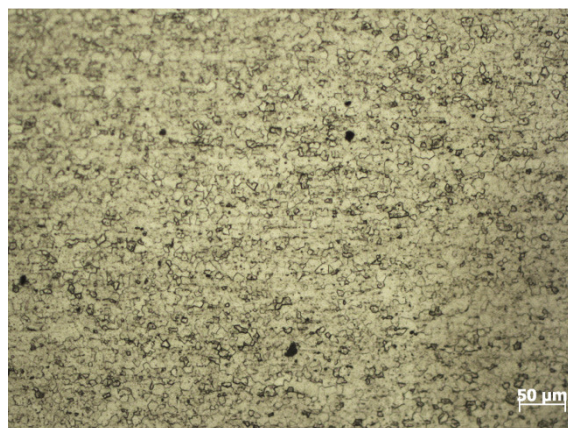
Fig. 3-2 – Microstructure of Ti-Fe-Si-O alloy
