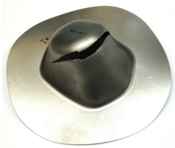
Fig. 4-15 – Deep drawing test on Ti-Al-Si-Nb
