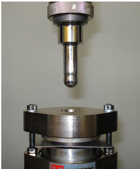
Fig. 3-29 – Erichsen test tooling
