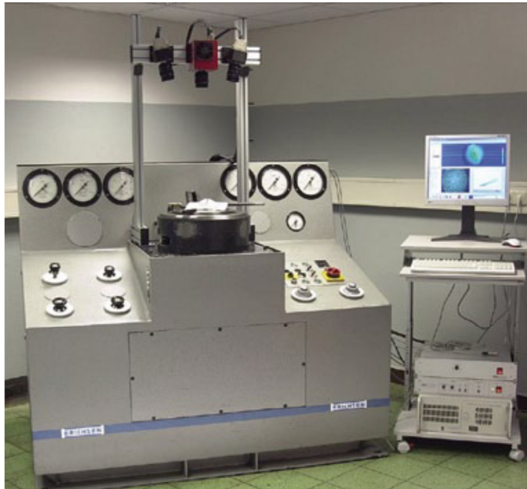
Fig. 5-6 – Testing equipment for Nakazima (or bulge) test
