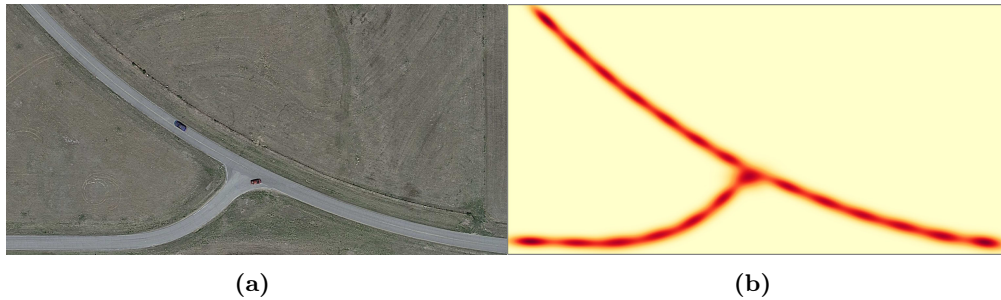
Figure 5.4: Test region: (a) Snapshot of the area from Google Maps; (b) heatmap of the calculated GMM, with darker colors corresponding to higher probability values.
