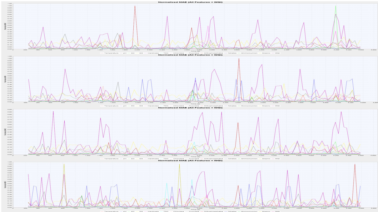
Figure 15: Normalized Mean Absolute Error (MAE) trends for all 12 features and WQI across the four RTUs during the complete experiment. Each panel corresponds to one RTU (top to bottom: RTU 1–RTU 4), showing real-time MAE evolution over all prediction rounds. The curves remain mostly stable with occasional spikes reflecting transient regime shifts or abrupt water-quality fluctuations.
