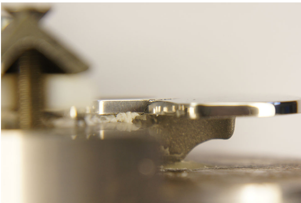
Fig. 9 Fatigue crack observed in the frontal plane
