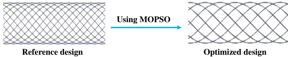
Figure 40. Comparative CAD design of the reference stent and optimized stent.
