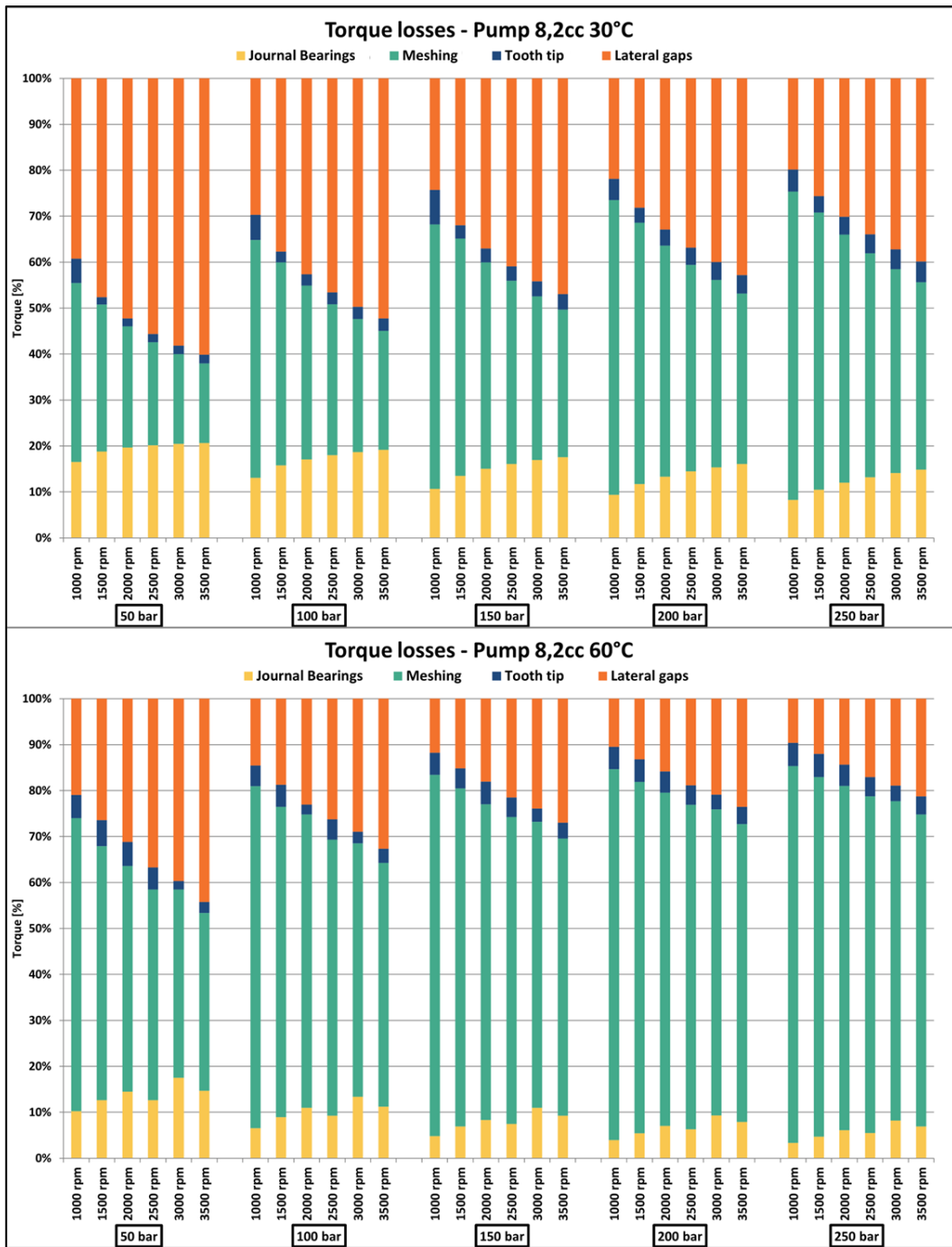
Figure 130 - Pump 8.2 cc No. 1 - Percentage contributions to torque losses at 30 °C and 60 °C
