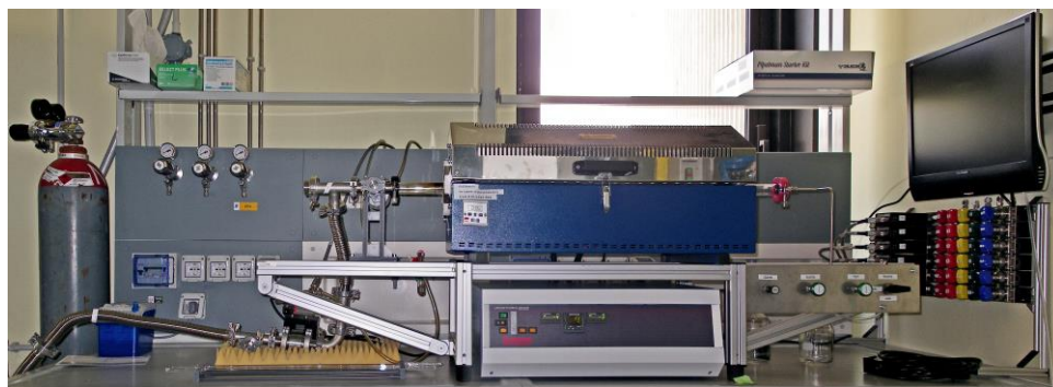
Figure S6. A Photo showing our furnace set-up used for the carbon coating and annealing experiments.
