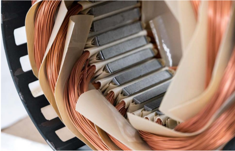
Figure 5.8 - Completed stator winding with PEEK magnet wire, PEEK slot insulation and PEEK phase insulation
