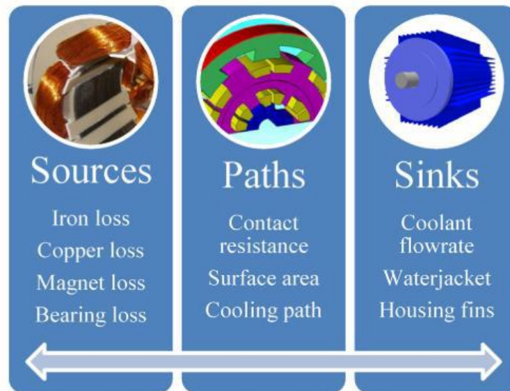
Figure 2.9 - Thermal management of electrical machines
