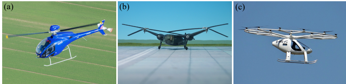
Figure 3.14: Examples of rotary wing VTOLs. a) Curti Zefhir [99] conventional helicopter; b) McDonnell XHJD-1 Whirlaway [100] side-by-side helicopter; c) Volocopter Volocity [29] multirotor
