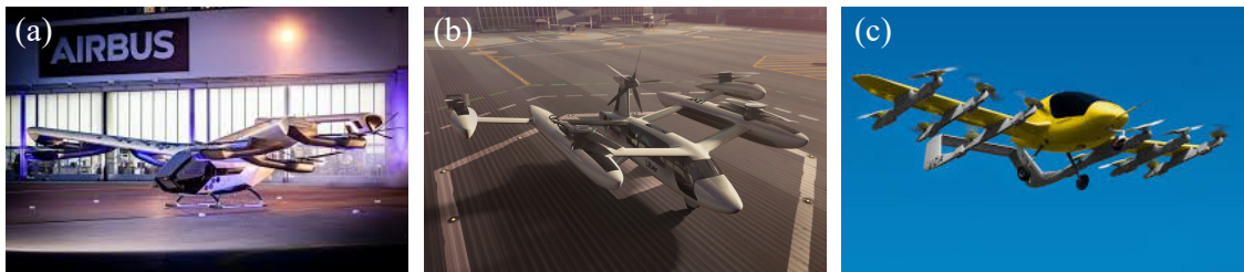
Figure 1.7: Lift+cruise VTOLs: AIRBUS NextGen (a) [36], Uber Elevate eCRM-003 concept (b) [39], Wisk 5 th Generation "Kitty Hawk" [38]
