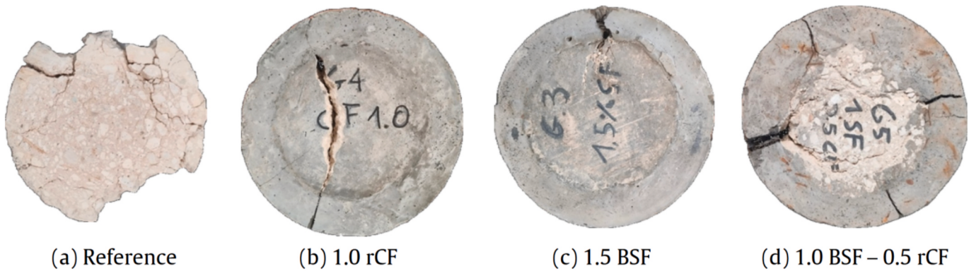
Fig. 19. Upper surface failure of concrete cylinders after compression tests.
