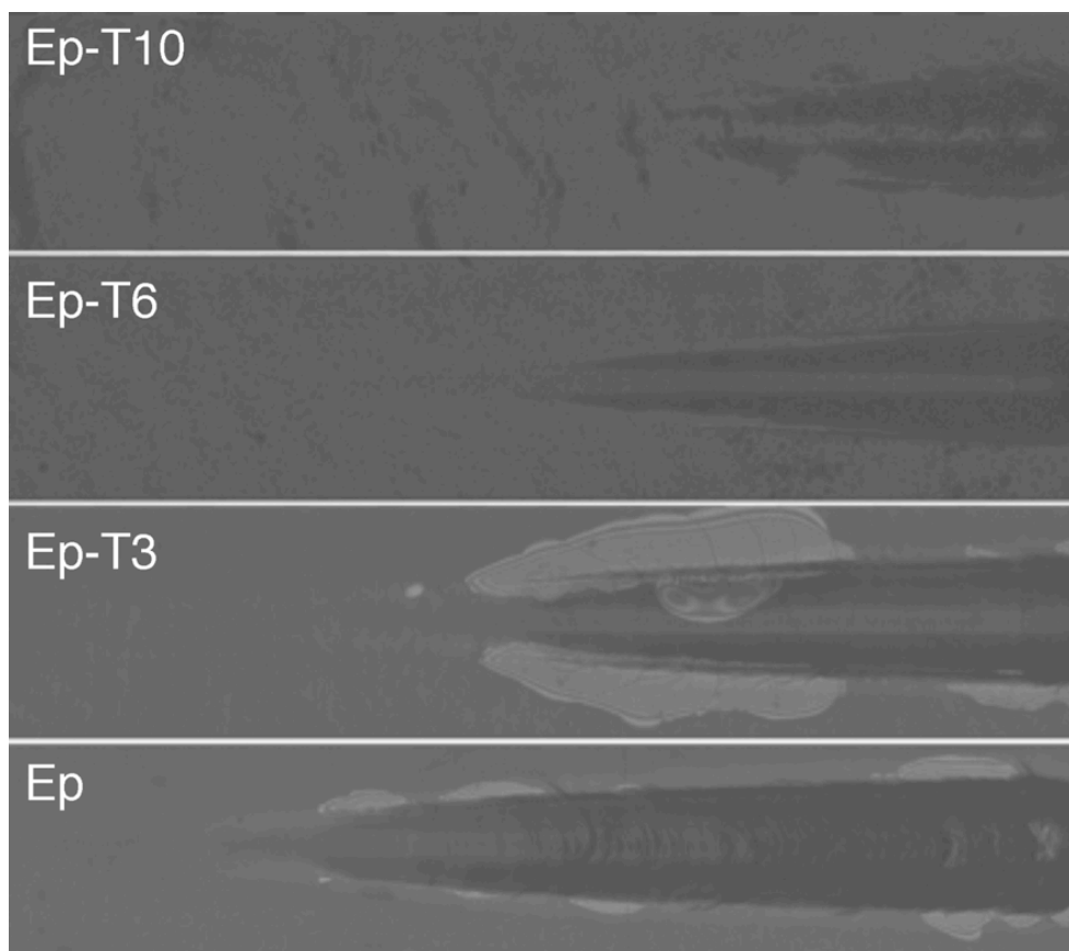
Figure 3.2.2.5 – Optical micrographs of the photo-cured coatings after scratch test (increasing load direction from left to right)
