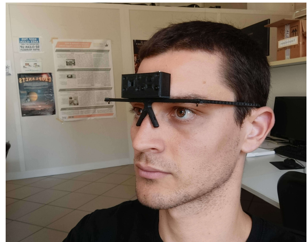
Figure 1. Complete system with all the sensors mounted on the glasses frame
