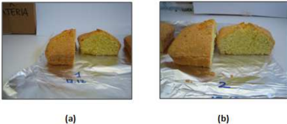
FIG 2.3 Test of leavening action (a) cake with REIBAKING POWDER (b) cake with the New Leavening Agent
