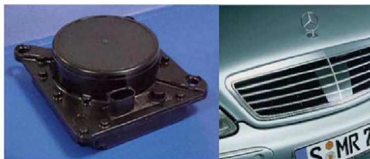
Figure 3.16: DISTRONIC radar sensor mounted on Mercedes Benz S-class vehicles.
