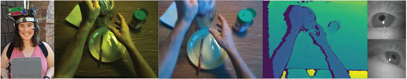
Figure 1: Left to Right: The device worn by a participant, highlighting the Ximea camera (blue), the Realsense D435i (red), the Realsense T265 (green), the Pupil Labs eye tracker (purple) and the operating computer (gray). Sample frames collected from Ximea camera, Realsense RGB stream, Realsense depth stream, and from the Pupil Labs binocular eye tracking cameras.
