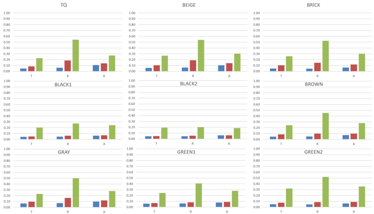
Figure 5.18 – Solar reflectance of glazed samples calculated according to ASTM E903 with AM1GH irradiance spectrum, divided for Uv-Vis-NiR wavelength range. The blue bar identify \rho_{UV} , red bar identify \rho_{vis} while green bar identify \rho_{NiR}
