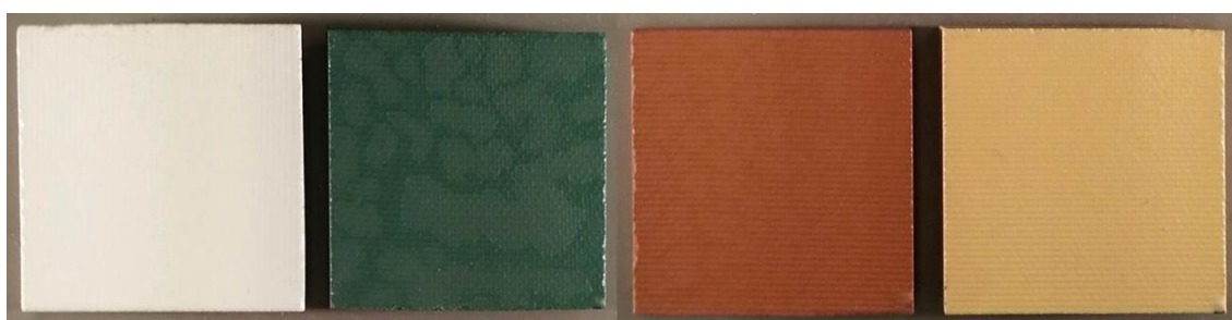
Figure 7.3 - Samples from Greece after accelerated ageing simulating (Arizona weathering conditions)
