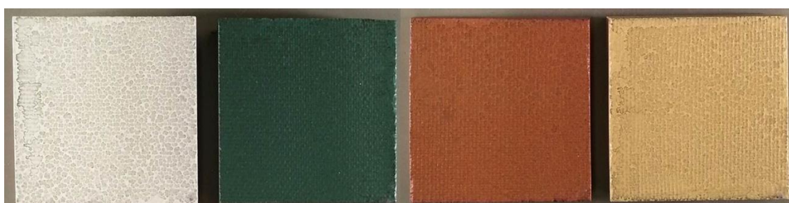
Figure 7.4 - Samples from Greece after accelerated ageing simulating (average weathering conditions)
