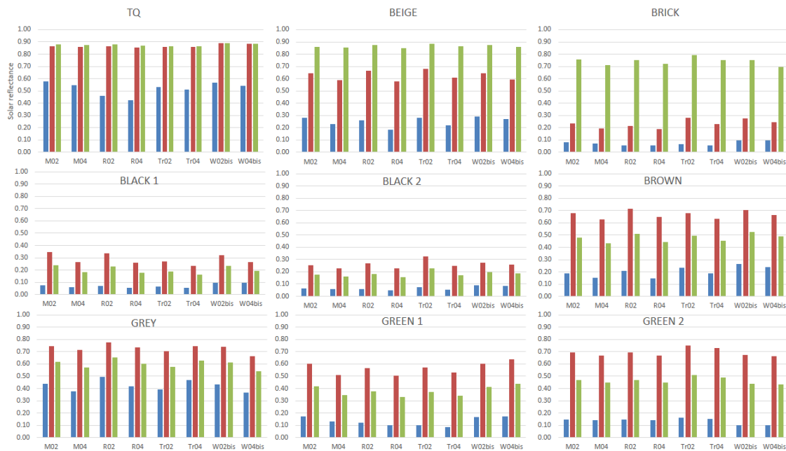
Figure 5.8 – Solar reflectance of the glazed samples calculated according to ASTM E903 with AM1GH irradiance spectrum divided for Uv-Vis-Nir wavelength range. The blue bar identify \rho_{UV} , red bar identify \rho_{vis} , while green bar identify \rho_{NiR}
