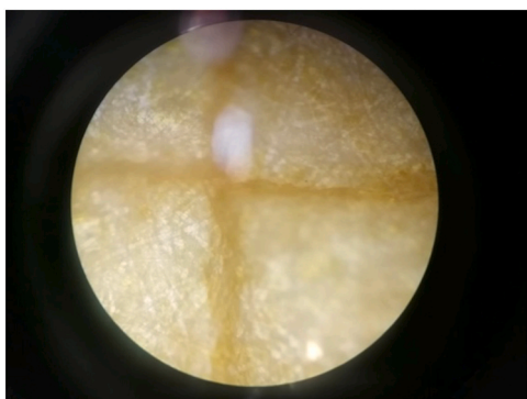
Fig. 7. Image of a PCL-cutin-coated paper sample after the folding test.
