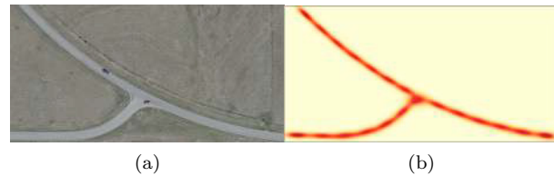
Fig. 4. Test region: (a) Snapshot of the area from Google Maps, (b) heatmap of the calculated GMM, with darker colors corresponding to higher values.
