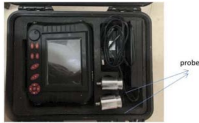
Figure 4. Ultrasonic instrument: WE-520 sound wave transmission detector (operating at 50 kHz).
