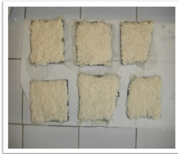
Fig.20. Stair step samples treated with the two different ethyl silicates.
