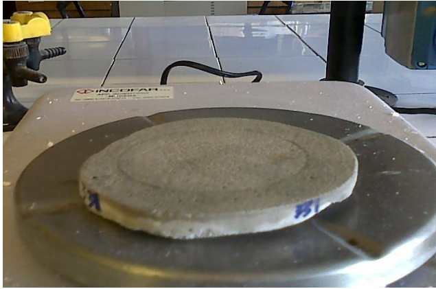
Fig.1. Penetration of the silicate visible on the edge of the sample.
