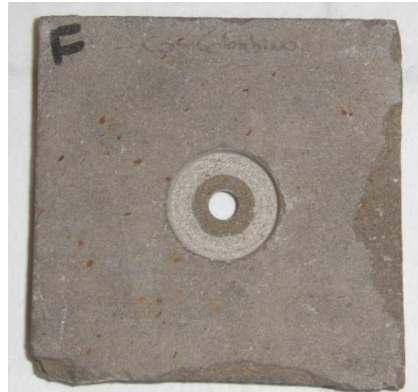
Fig.18. Colombino heat-treated with trace of disaggregation (on right and bottom side).
