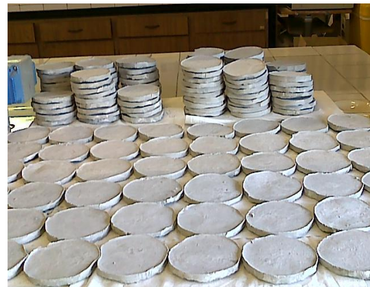
Fig.20. Drying step of artificial test pieces.
