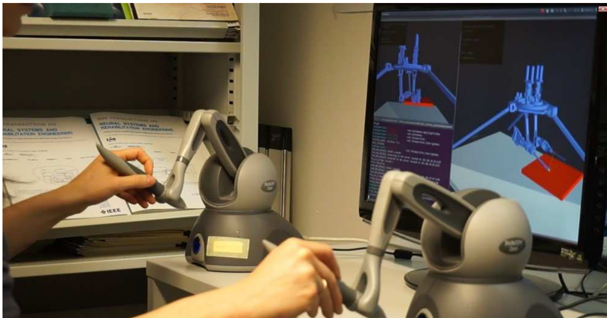
Figure 4.37: Teleoperation of the two arms of the I-SUR robot.
