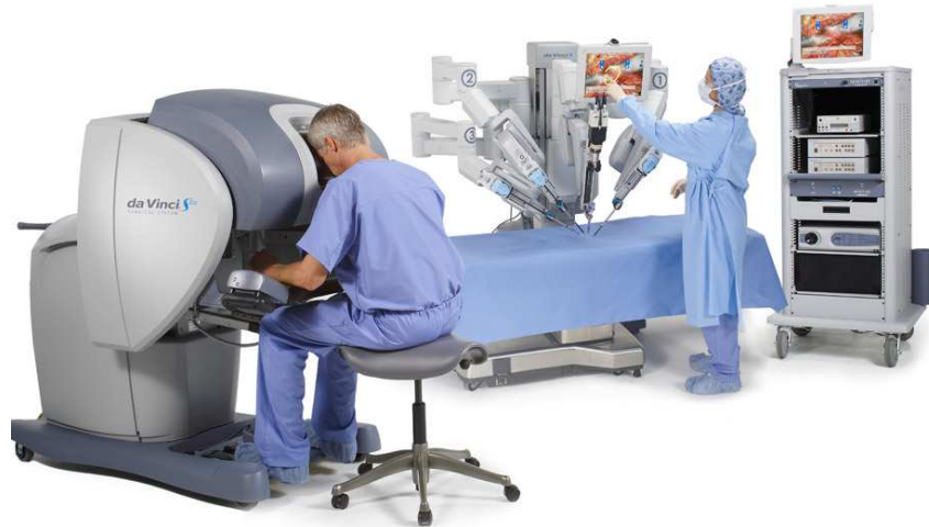
Figure 1.1: The Da Vinci surgical system with its surgeon's console (left) and the robot arms (right).
