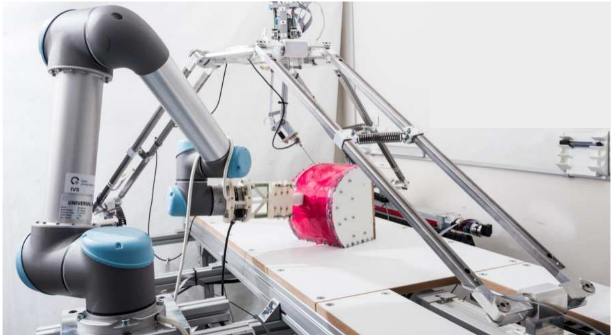
Figure 4.4: The overall robotic platform for needle insertion. On the left, the UR5 robot holding the US probe; on the right, the I-SUR robot holding the needle; on the operating table, the phantom of the human abdomen.
