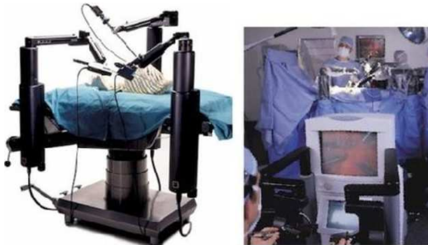
Figure 1.2: The Zeus surgical system with its table-mounted arms (left) and the surgeon's console (right).
