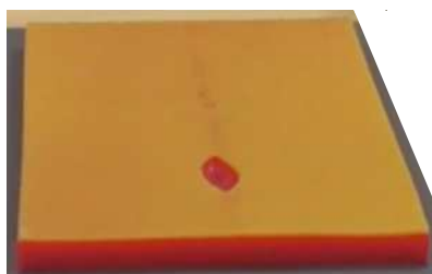
Figure 4.29: Suturing pad reproducing the cutaneous (yellow) and subcutaneous (red) layers of the human abdomen.
