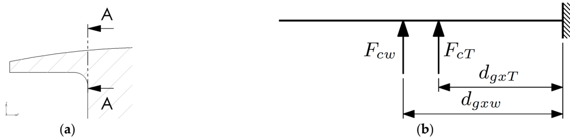
Figure 3. Section A-A: the crossbar of the T-shape: (a) detailed view; (b) analytical model.
