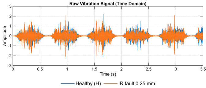
Fig. 1. Vibration signals were obtained from an accelerometer affixed to the guide rail during a single bidirectional traversal of a curved module under both healthy (H) and inner-race fault (IR 0.25 mm) conditions. These signals demonstrated pronounced amplitude modulation due to the acceleration, steady motion, and deceleration phases. The impulses associated with faults are obscured by variability induced by motion and are not consistently discernible in the time domain.
