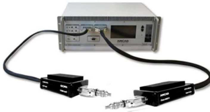
Figure 4.20: Picture of the AMCAD 200 Pulsed IV system used for the characterization.
