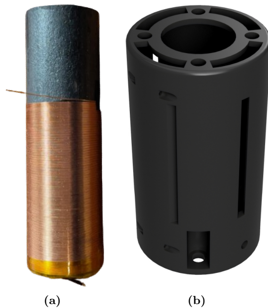
Figure 3.22: Electromagnetic gripper composed of: (a) a conductor wrapped around the electromagnetic core and (b) a plastic tool shell.
