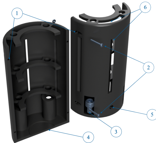
Figure 3.24: Render view of the gripper shell, with key features: (1) Assembling through-holes, (2) M2x15 assembling screws, (3) Mounting M6 screws and notches, (4) Shell flange, (5) Through-hole for cables, and (6) Radial and axial cuts for thermal dissipation.
