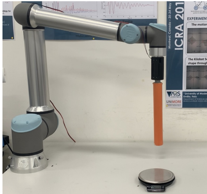
Figure 3.25: Test for the maximum grasping mass with sample of 1500 g.
