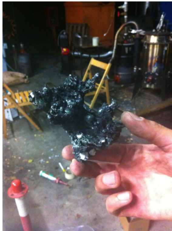
Figure 8.11: Melted ashes found in the stratified reactor
