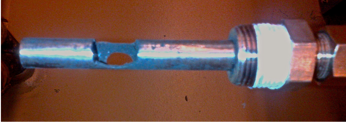
Figure 6.14: fouling of the inlet tube
