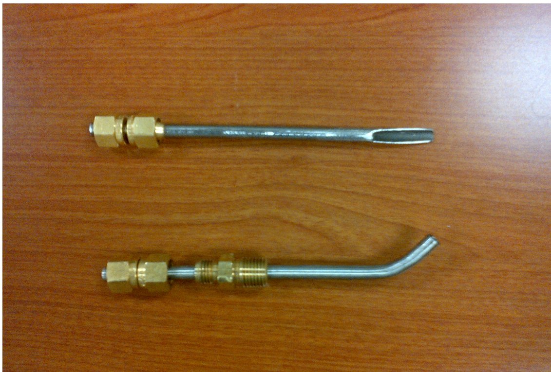
Figure 6.10: Two solutions designed for separation of 1/10 of the gas stream
