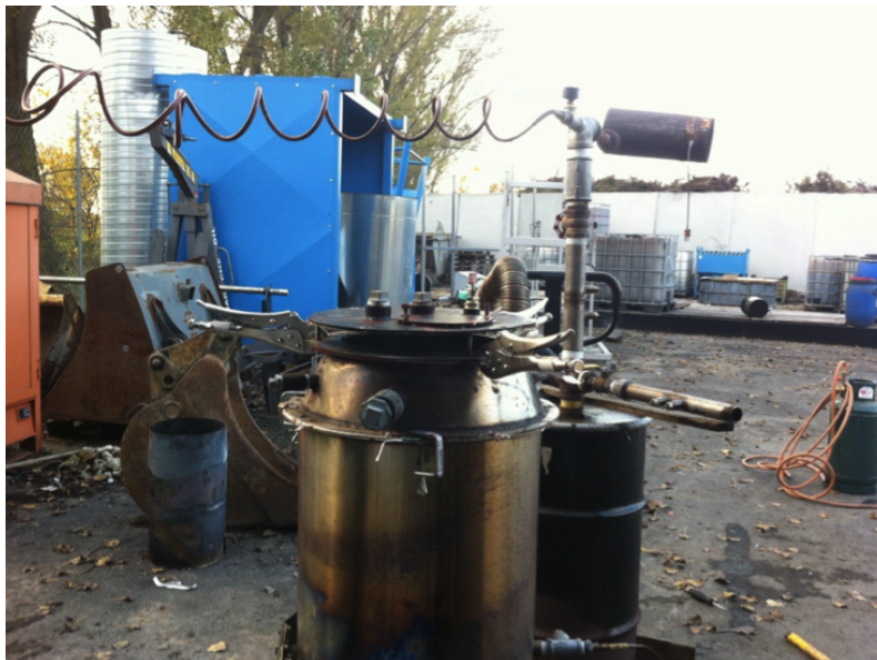
Figure 8.8: Stratified reactor obtained from G.E.K.
