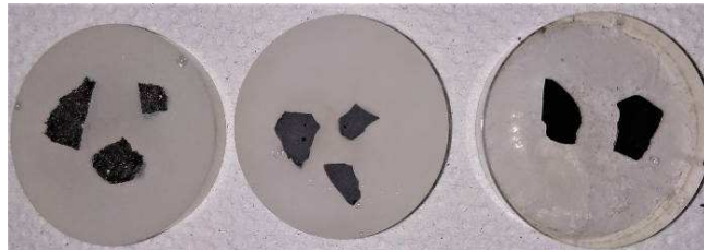
Figure 3.1 - Mounts showing the three different polishing steps.
