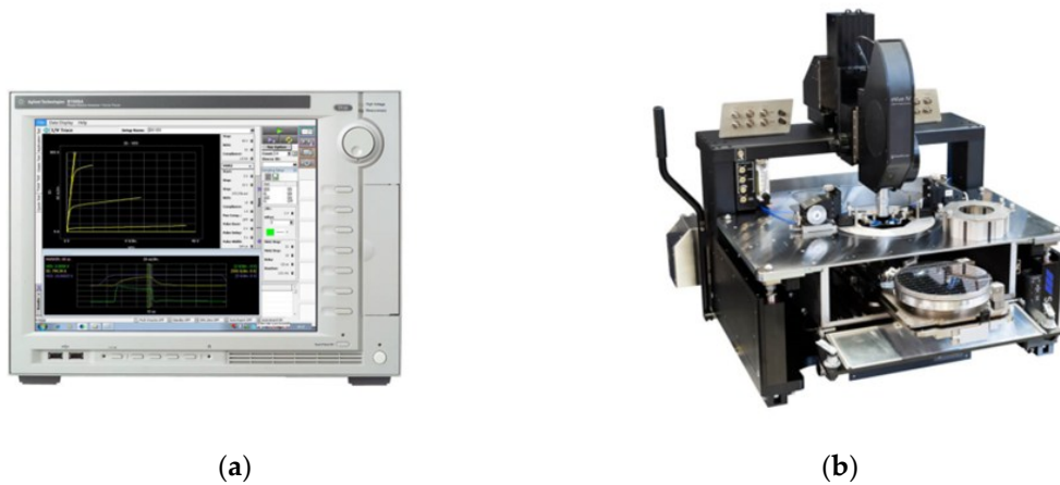
Figure 4.13: (a) B1505A parameter analyzer; (b) Probe system for on-wafer measurements.
