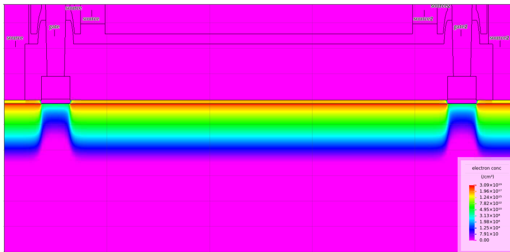
Figure 5.21: TCAD simulation of the 2D electron concentration of the bidirectional DUT in off state (zero source-to-source voltage).
