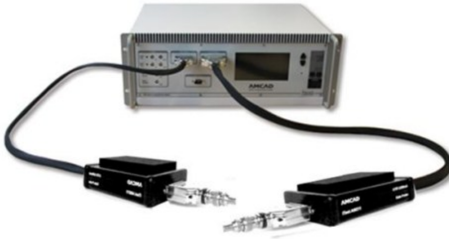
Figure 3.5: AM200 system for evaluation OTF PIVs.
