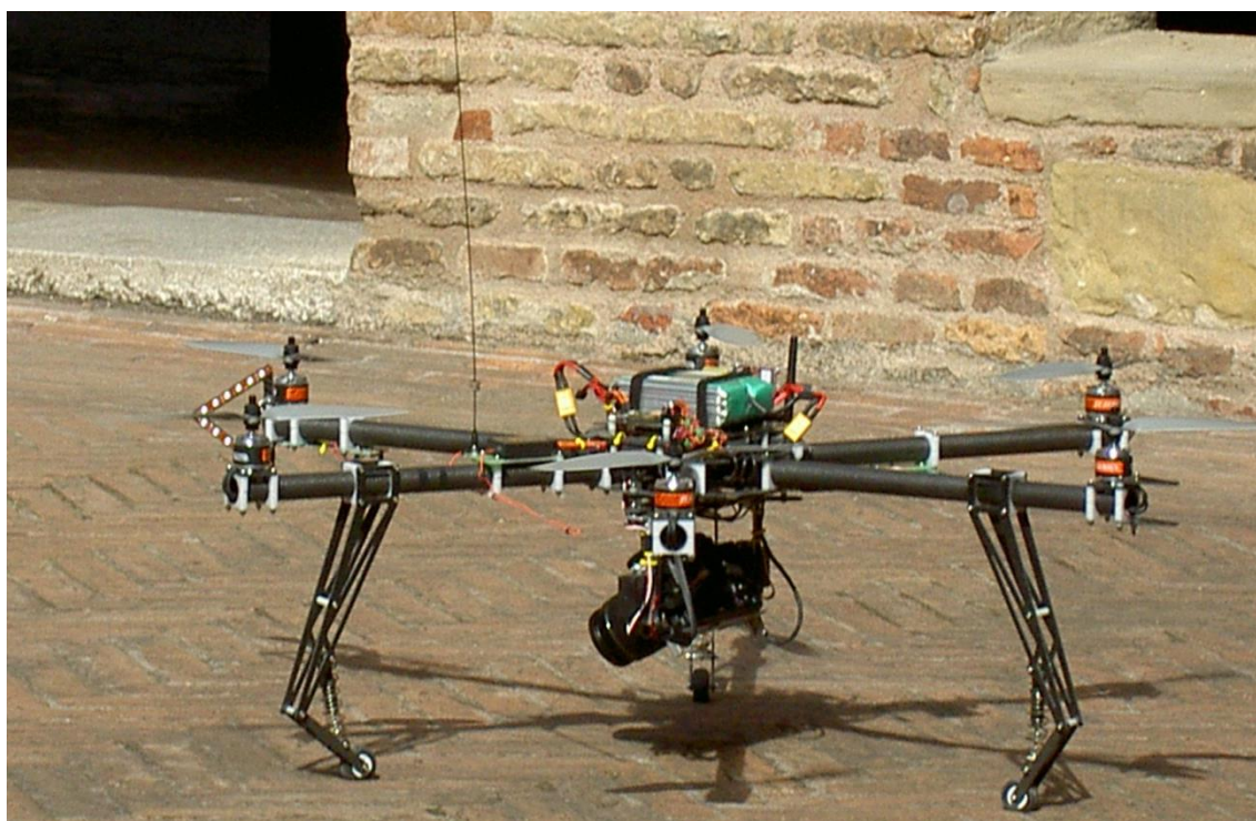
Figure 7.4 The UAV Hexacopter with the embedded equipment
