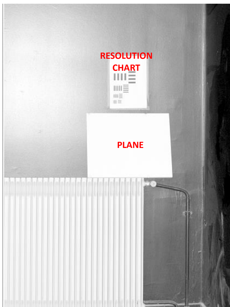
Figure 6.28 The best-fitting and optical resolution estimation experimental test
