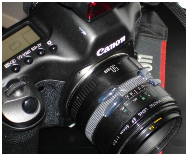
Figure 6.44 Canon EOS 5D and the glued lens
