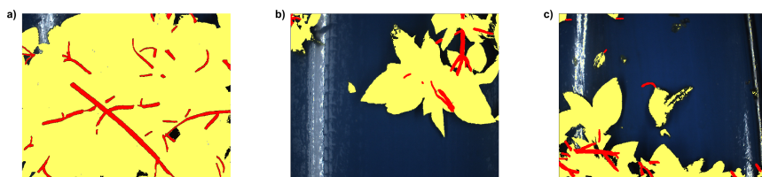
Figure 4.2 – Labeled images used for training the classification model where red pixels represent branches, yellow pixels correspond to stems.
