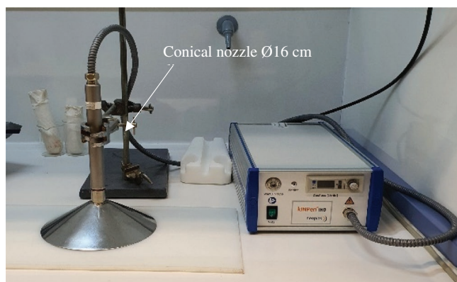
FIGURE 1 | Configuration of the kINPen IND system with the attached conical nozzle. [Color figure can be viewed at wileyonlinelibrary.com ]
