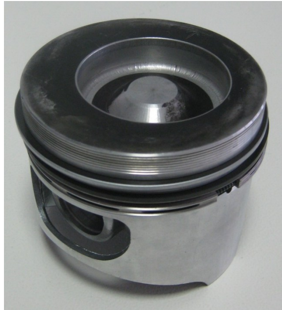
Figure 8: Modified piston bowl for hydrogen operations [68].
