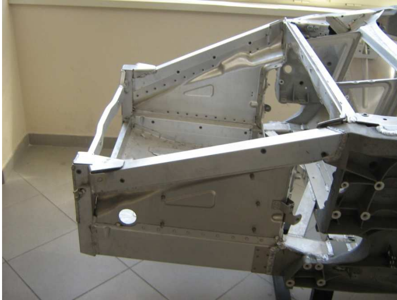
Fig.2.2 front crumple zone of a Ferrari F430.
