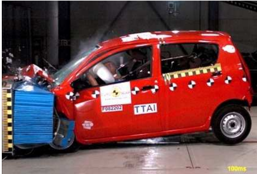
Fig. 1.2. Daihatsu Charade NCAP frontal offset test with a deformable barrier.
