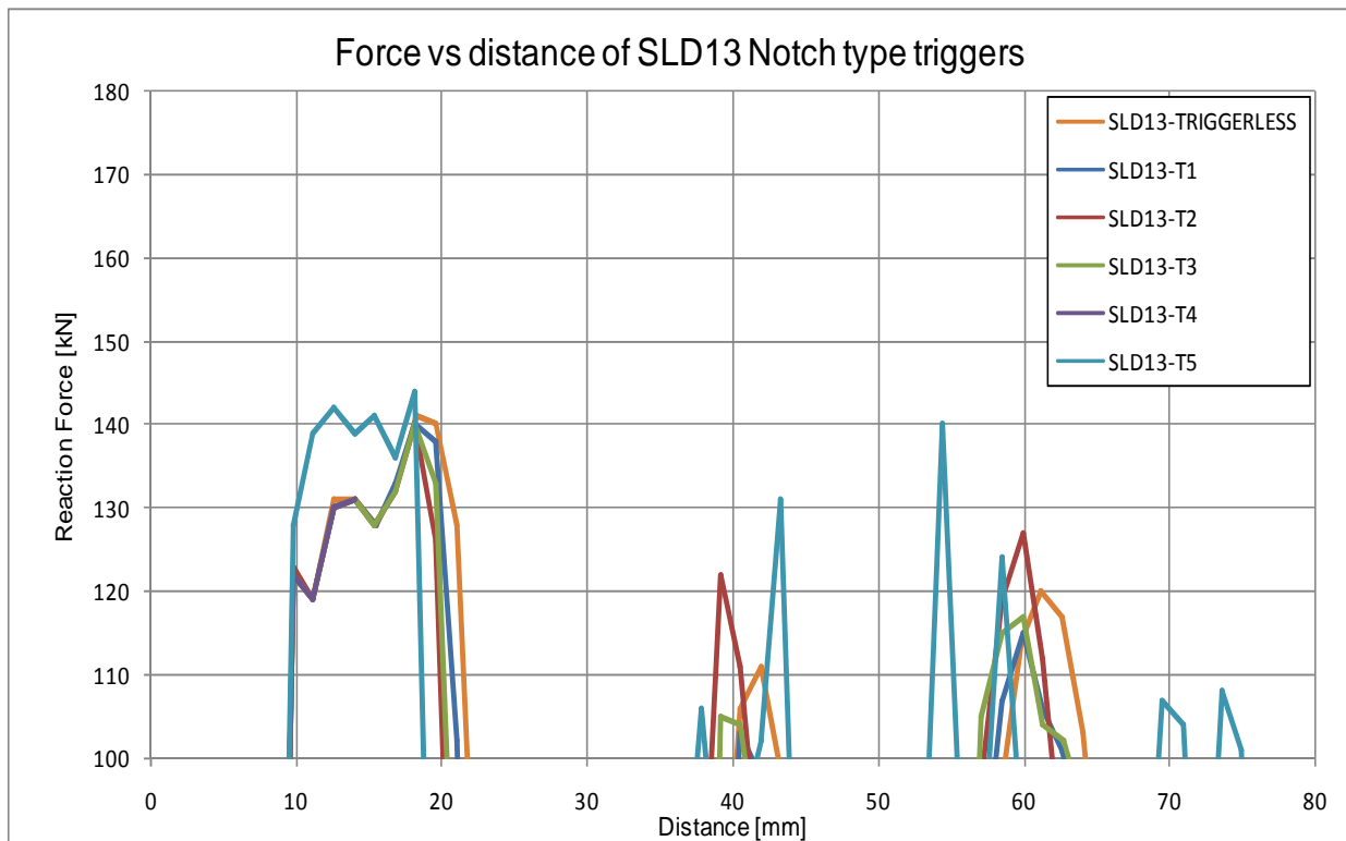
Fig. 4.4. Comparison of different triggers for SLD13 Force vs. displacement curves.
