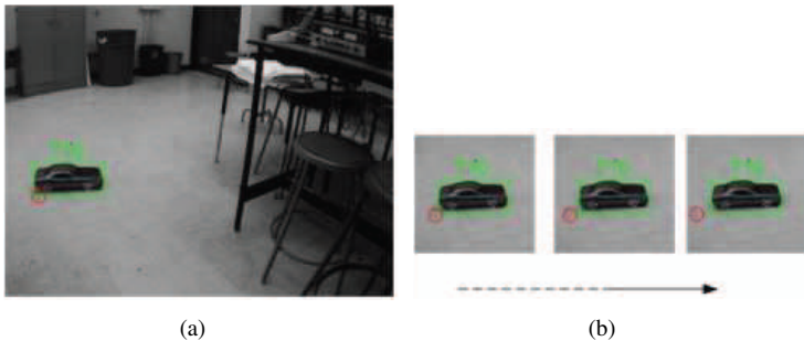
Figure 6.18: Last QVGA frame captured while computing pixel displacement of tracked object (a), and Search regions cropped at hardware level (b).
