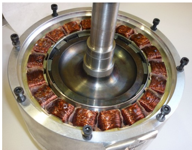
Figure 1.1: Example of an inner rotor synchronous permanent magnet machine.
