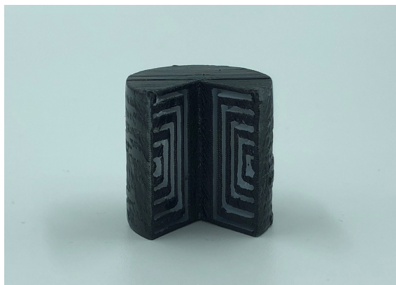
Figure 4.1: Additively manufactured mock up prototype of the plunger pole of the synchronous tubular machine with five layers [14].
