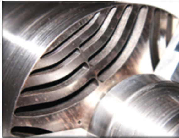
Figure 5.2: Example of a pure reluctance rotor.
