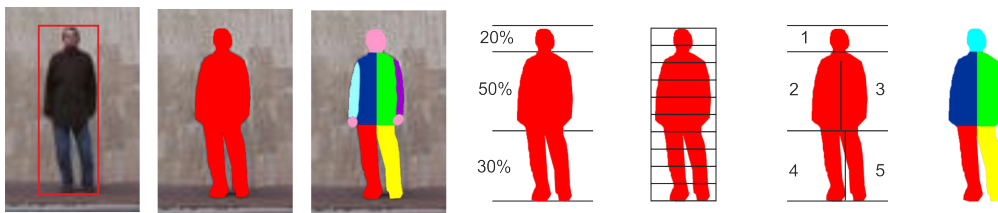
Figure 2.2: From left to right: Region of Interest: bounding box by people detection, complete pixel-wise silhouette from foreground segmentation, face/body part segmentation and classification. Examples of body models: three horizontal fixed slices [5, 123, 160], ten slices [34], symmetry based parts [80], five human body parts [19]
