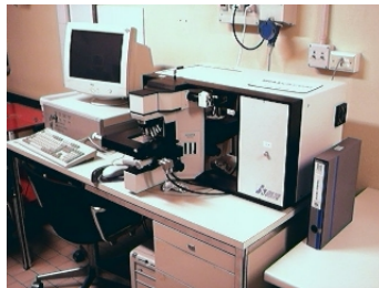
Figure 2.13: LabRam Horiba Jobin Yvon at the CIGS labs in Modena.
