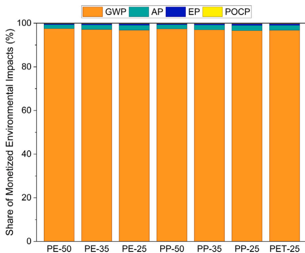
Fig. 5. Relative contribution of external (environmental) costs per impact category for each SHLC 4 formulation under the maximum valuation scenario.
