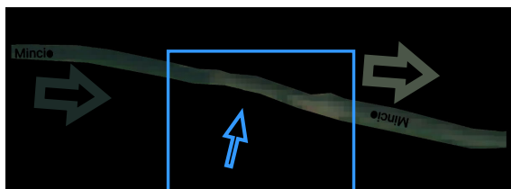
(d) The river color turns lighter because of the high-turbidity tributary. Only by masking the background, it becomes evident
