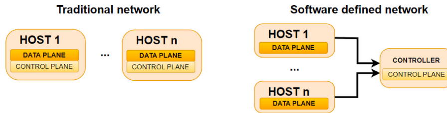
Fig. 5. Traditional network vs. Software defined network.
